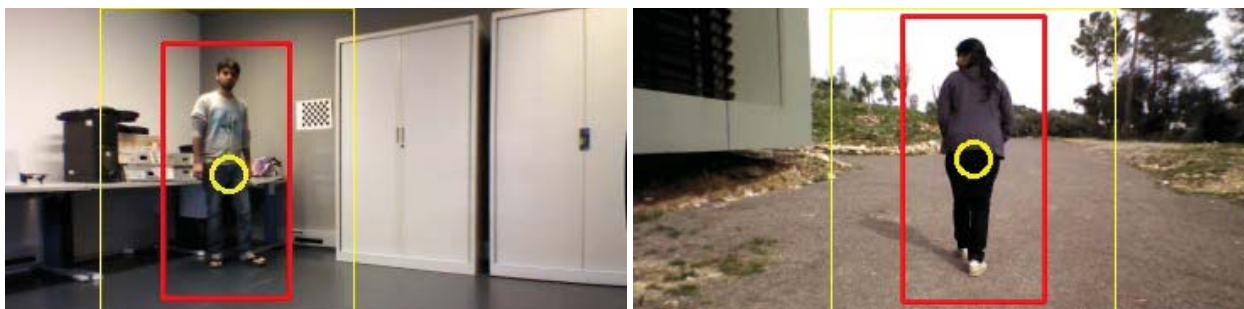
Figure 4: Tracking a person. On the left picture, a HOG transform is used to detect a region of interest. In the right picture, a particle filter is used in the region of interest to know whether the same person is being followed.
